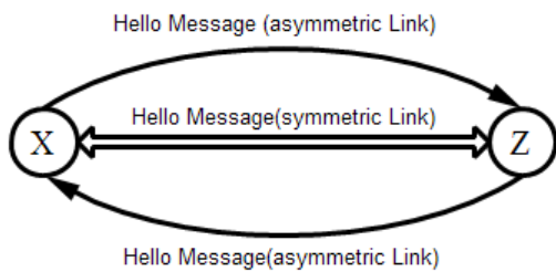
Fig.4 OLSR Symmetric link formation (Hello Message Exchange)
