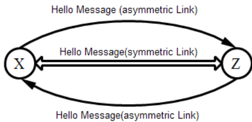
Fig.4 OLSR Symmetric link formation (Hello Message Exchange)
