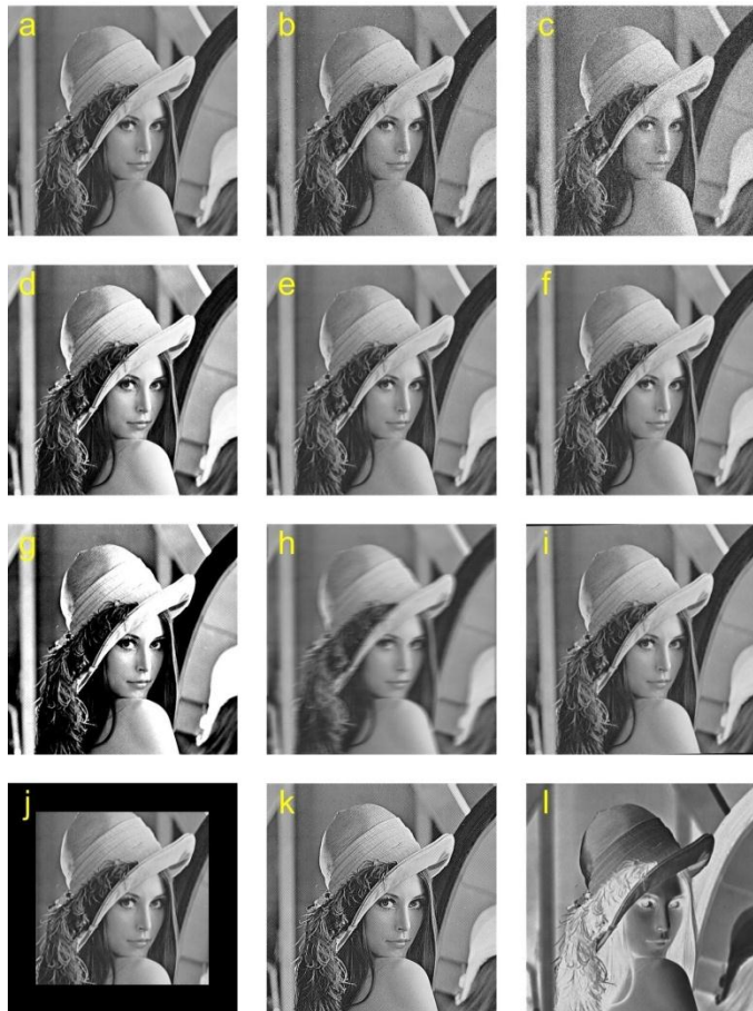
Fig.8. Watermarked Image under different attacks : (a) JPEG compression, (b) Salt & pepper noise 10%, (c) Gaussian noise [0,0.01] (d) Histogram Equalization, (e) Median filter [3×3], (f) low-pass filter [5×5], (g) Gamma correction 0.6 (h) motion blur 45°, (i) Rotation (1°), (j) Cropping (25%).
